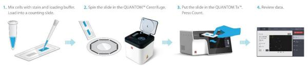
Counting with the QUANTOM Tx Microbial Cell Counter
