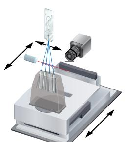
The angle and the position of the side streams are calculated and adjusted during setup for tube and plate sorting. This ensures that the sort stream is centered in the collection tube automatically.
