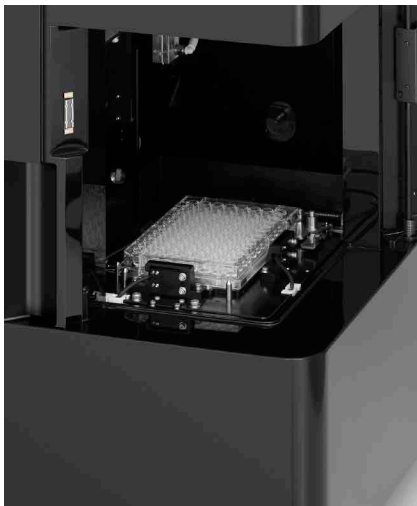
Figure 4. Plate motion uses a fixed probe and moves the plate (and sample) in horizontal and vertical directions.
