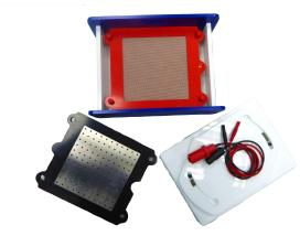
The BlueBlot Semi-Dry Blotter consists of a spring-mounted anode, a drill holes carrying cathode made from stainless steel. The housing is closed with the lid and secured by a newly developed rotating device mechanism. Due to the design of the cable pins wrong connection is excluded.
