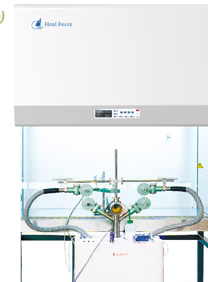
KI-discus containment test 2
